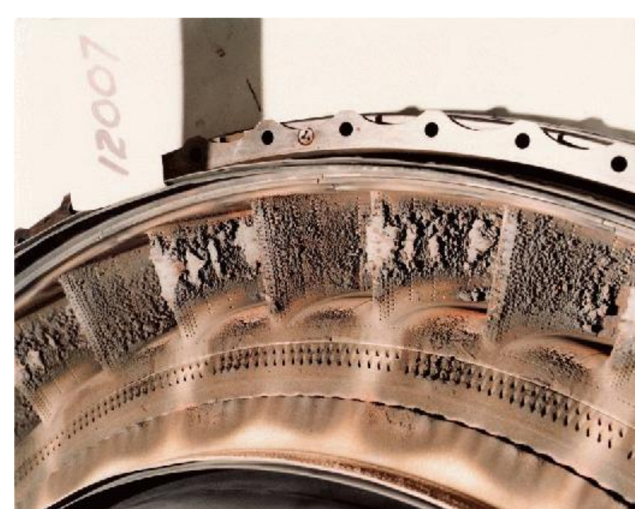
Figure 2. British Airways engine after a run in with a volcanic ash plume, 1982
